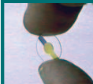
Figure 3. A quartz crystal containing gold electrodes
